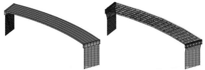
Figure 4. Undeformed and deformed shape of a curved integral abutment bridge with 400 ft radius and 4 to 50 ft spans with 28.65° of curvature with piles in very stiff clay soil profile with 9 ft deep predrilled holes filled with loose sand. The bridge is subjected to a thermal load of \Delta T_{\text{slab}} of 120° F and \Delta T_{\text{the rest}} of 90° F. A deflection scale factor of 40 is used to enlarge the displacement of the bridge structure.
